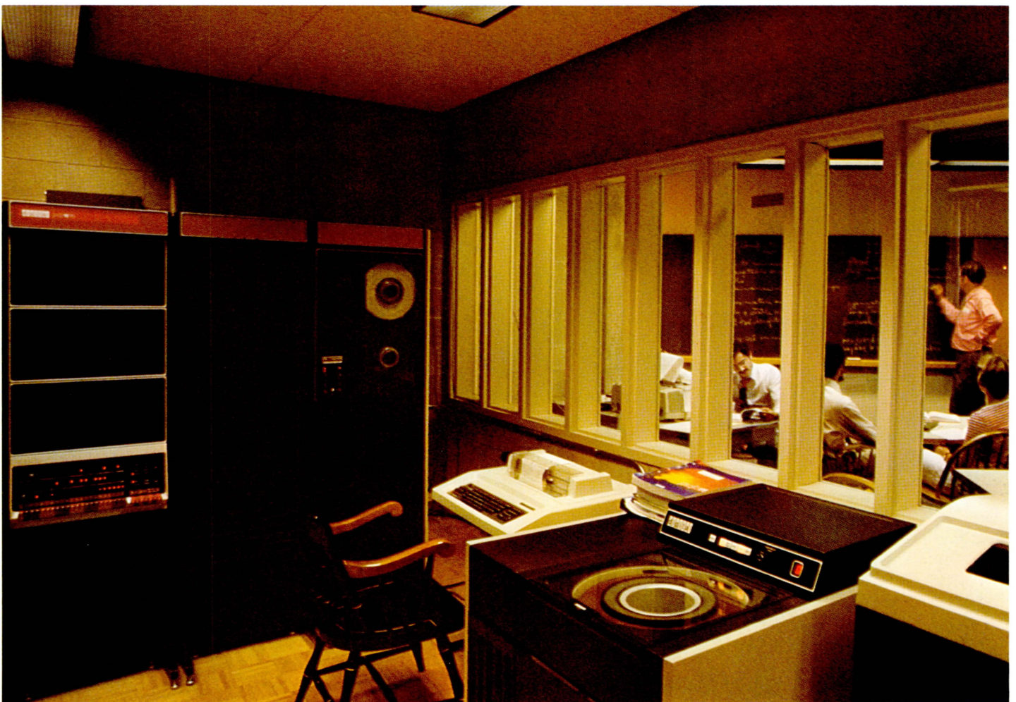
A Digital PDP-11/70 system at Babson College in Wellesley, Mass. serves as the central computer for a consortium of local colleges and universities, performing a variety of academic and administrative data processing tasks. Babson uses the system for student registration, class scheduling, grading and alumni record-keeping and student billing, in addition to the classroom instructional use shown here.
