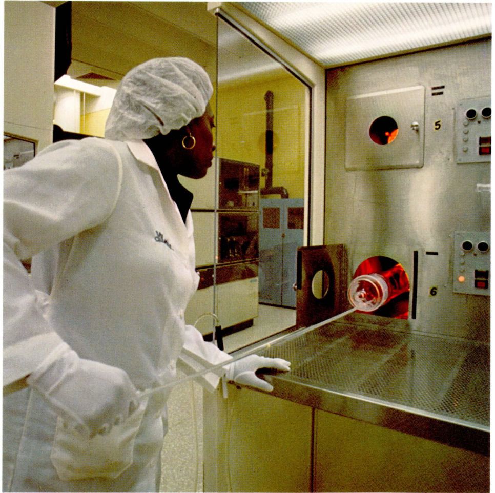
At Digital's semiconductor development facility in Worcester, Mass., silicon wafers are placed into a diffusion furnace to "grow" oxide on the wafer surface. Microscopic circuitry is then achieved on each wafer by means of a photographic masking technique. Each 3-inch wafer has the potential for up to 200 microcircuits. After testing, each circuit is packaged, retested and placed on modules to form the heart of Digital's LSI-11 microcomputer.
