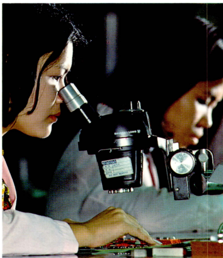
More than 20 billion bits of core memory are produced at Digital's facilities at Taiwan and Hong Kong. Here, inspectors at Taiwan perform microscopic quality assurance on memory arrays.
