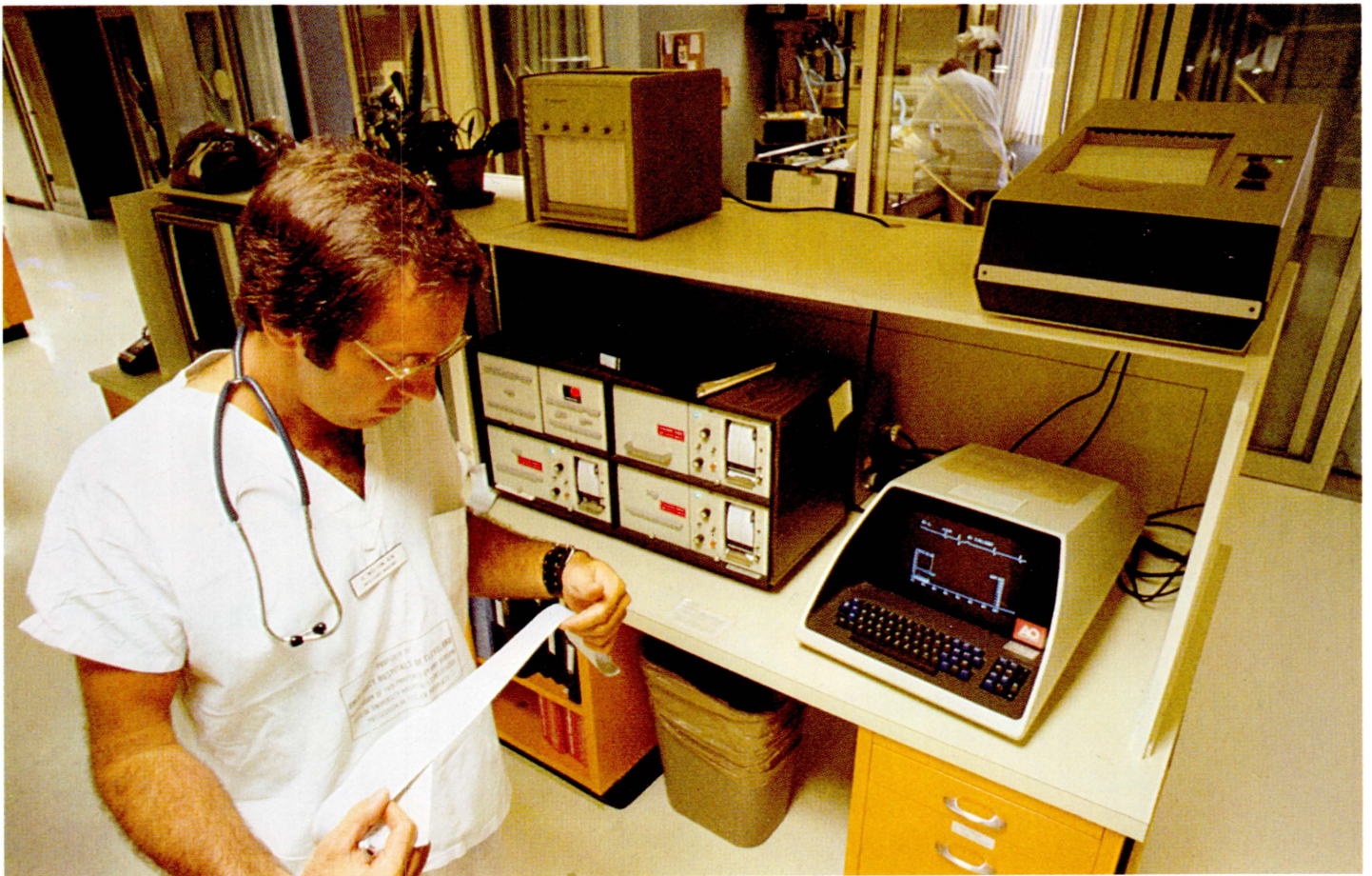
Patients in the Medical Intensive Care Unit at University Hospitals of Cleveland, Ohio are under the watchful eye of a bedside monitoring system which transmits heart rate, blood pressure and other vital signs to a central station where it is displayed on a Digital video terminal controlled by a PDP-11 computer. The system, designed by American Optical Corporation, monitors up to 20 patients simultaneously. It can provide immediate information on any patient and sounds an alarm if a medical emergency develops.
