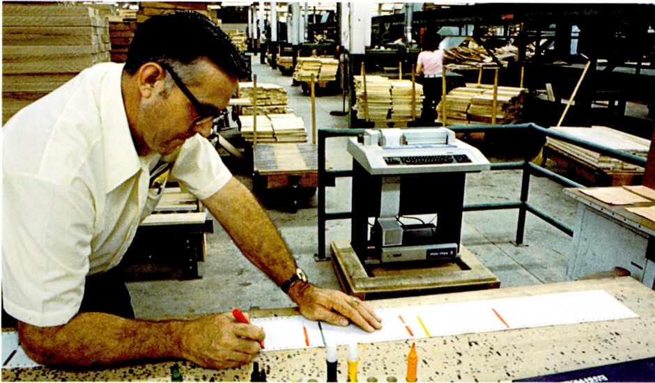
Trim loss of expensive hardwood used in the manufacture of fine furniture is kept to a minimum at American Drew Furniture Company factory in North Wilkesboro, North Carolina. A special system developed by Barr-Mullin, Inc. uses a small Digital PDP-11 computer located on the factory floor to compare furniture design to characteristics of the board being cut to determine the most efficient cutting pattern. A Digital LA36 DECwriter located with the PDP-11 prints out the computer's analyses.
