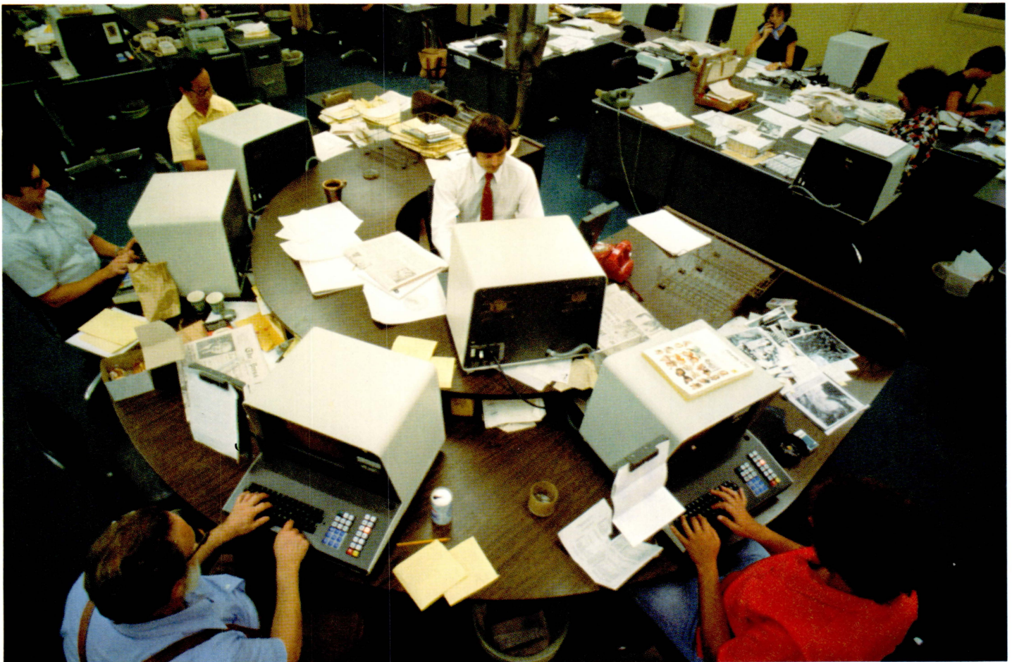
Reporters and editors at THE PRESS, a daily newspaper serving southern New Jersey, use Digital VT20 graphics terminals instead of typewriters to speed news to their readers. Stories are written, edited, and sent directly from the terminals into a large Digital PDP-11 system which controls justified typesetting and production of copy which is ready for printing.
